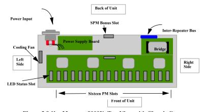
Figure 3.9.1b: Magnum 8000X, Top View with Chassis Cover
